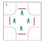
**Current Signal Progression:** Pedestrians must "apply to cross" by pushing a button and often have wait for up to four signal phases before crossing.
