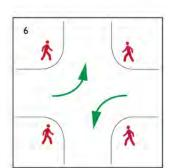
**Proposed Signal Progression:** Pedestrians and vehicles get a concurrent green signal. Pedestrians get a 3-second head start (leading pedestrian interval) to prevent being hit by right-turning vehicles.
