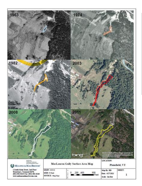
**Figure 12.** This series of maps shows how the MacLauren Gully began in 1963 and has continued to erode and expand significantly in the last 50 years. This project resulted in the first of its kind in Vermont landslide hazard map.
