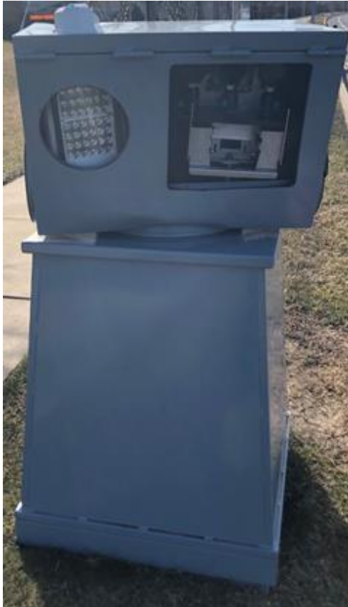
Figure 11 Camera System with Box Enclosure
