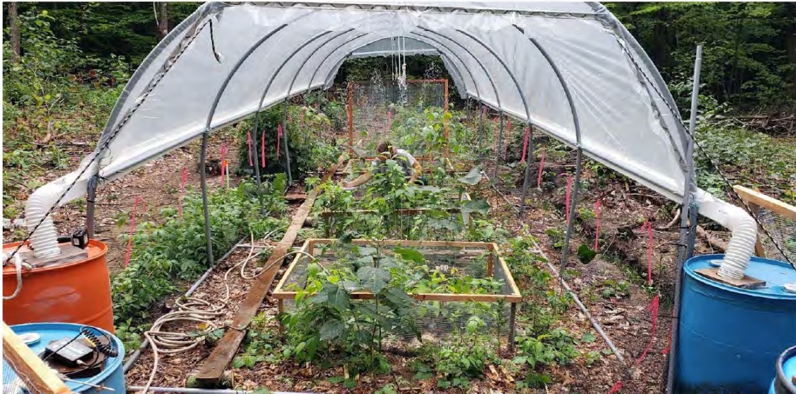
Figure 2-14: Experimental plots (elevated wooden rectangles) within a forest gap with controlled precipitation (exclusion, watering) used in the forest regeneration precipitation manipulation experiment at the University of Vermont Jericho Research Forest. Photo: Peter Clark
