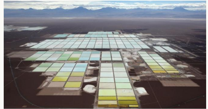
Brine pools at the Soquimich lithium mine on a salt flat in northern Chile. IVAN ALVARADO / REUTERS VIA ALAMY
