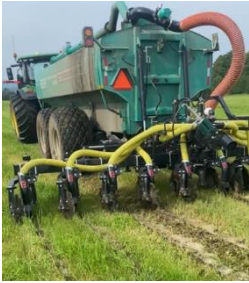
Figure 14: Grassland Shallow Slot Manure Injection equipment is a very shallow manure injection method which causes a low level of soil disturbance. This application method significantly reduces surface phosphorus application and nutrient loss while increasing efficiency and crop production. This equipment purchase was funded through the Vermont Agency of Agriculture, Food & Markets Capital Equipment Assistance Program.
